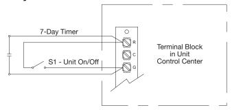
For 7-Day Timer, use blue and black wires. Red wires should be capped off.
